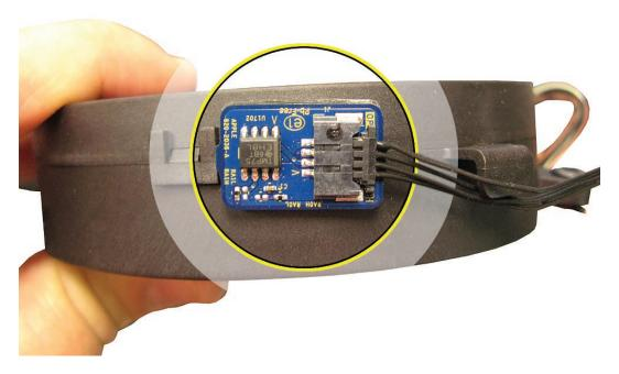
2. Lower the fan into the rear housing. Press the foam gasket into place across the top of the fan.
